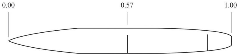
Figure 1 Planform View of Model Configurations Tested (adapted from Berrier (1994)). Dimensions are in Fractions Of Body Length (L)
